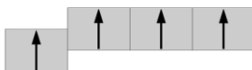
Fig. 3. Graphical formula external electronic energy level of carbon atoms in the excited state
