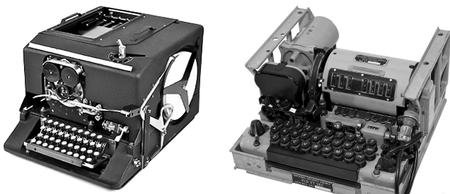
Figure 1.13 – American rotary encryption machines SIGABA (ECM MARK II) and its successor KL-7 9
