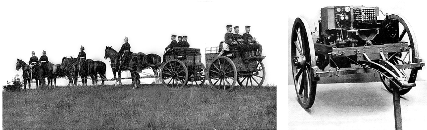
Figure 1.8 – Horse small (field) military radio station with a combat crew of the early XX century
