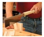
Finger pointing. An alternative is to extend the index finger along the length of the handle to help direct the saw.
