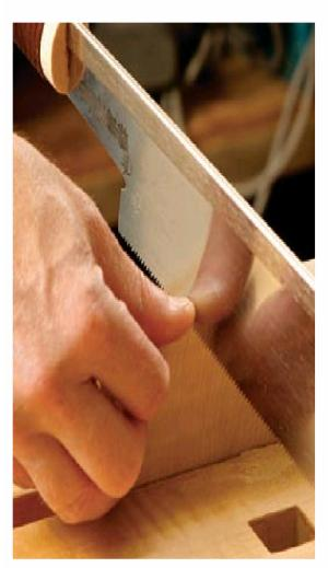
**Guide the cut with your thumb.** Angle the saw very slightly and start cutting at the back corner. Use very light cuts and let the teeth do the work.
