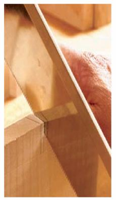
Back out and try again. If you find that the cut has drifted off course, don't try to correct it by tilting the saw; the thin blade will bend. Instead, back the blade out and start again at a steep angle until you are back on the right line.
