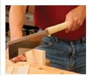
**End of the handle.** Durfee prefers to hold the saw near the end of the handle for a light touch.
