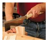
Tuck the handle in. Some users prefer to hold the handle close to the blade and keep the end of the handle close to their side to help guide the saw.
